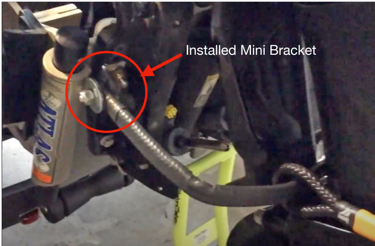
Figure S1-10: Installed Mini Bracket for The Leash
