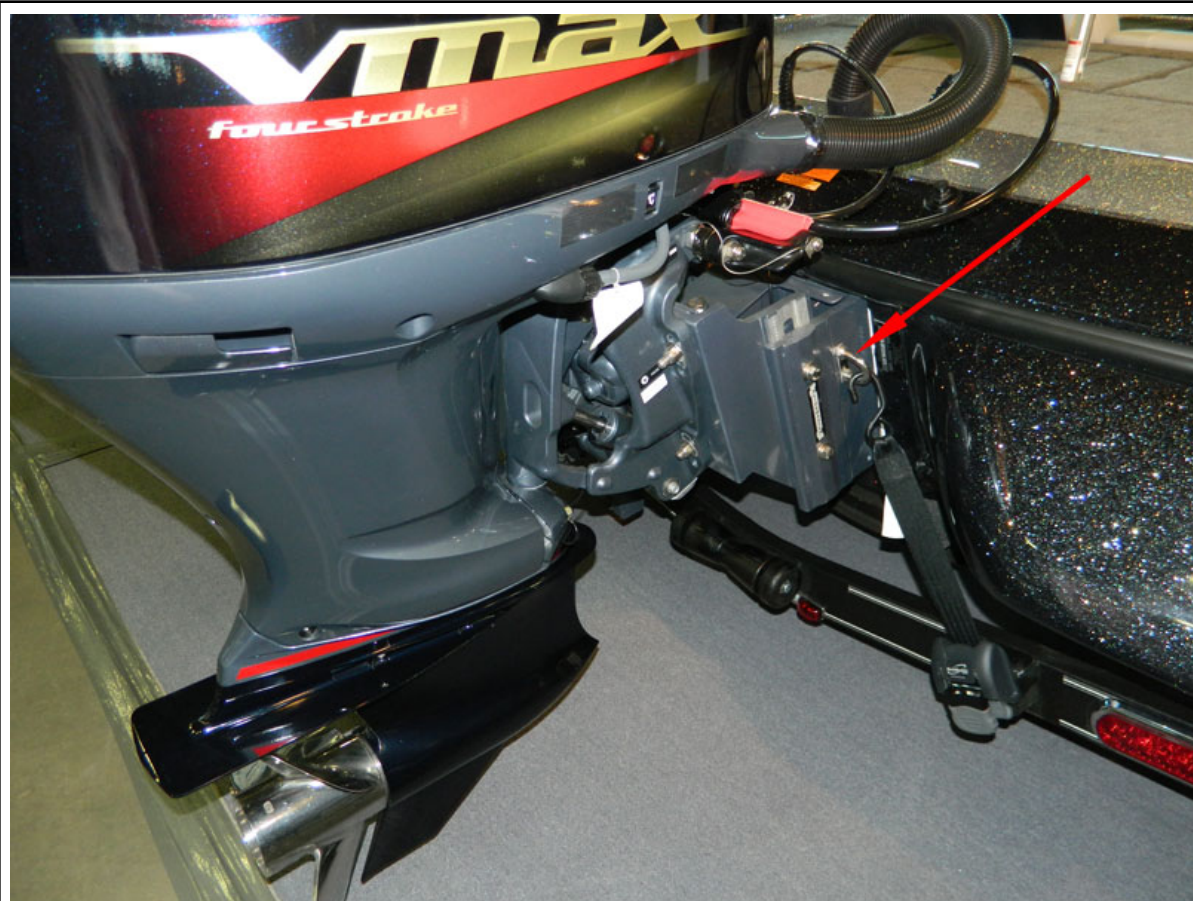
Figure 43: Yamaha 250 VMAX SHO on Slidemaster Jack Plate with U-bolt tie down behind a Skeeter boat
