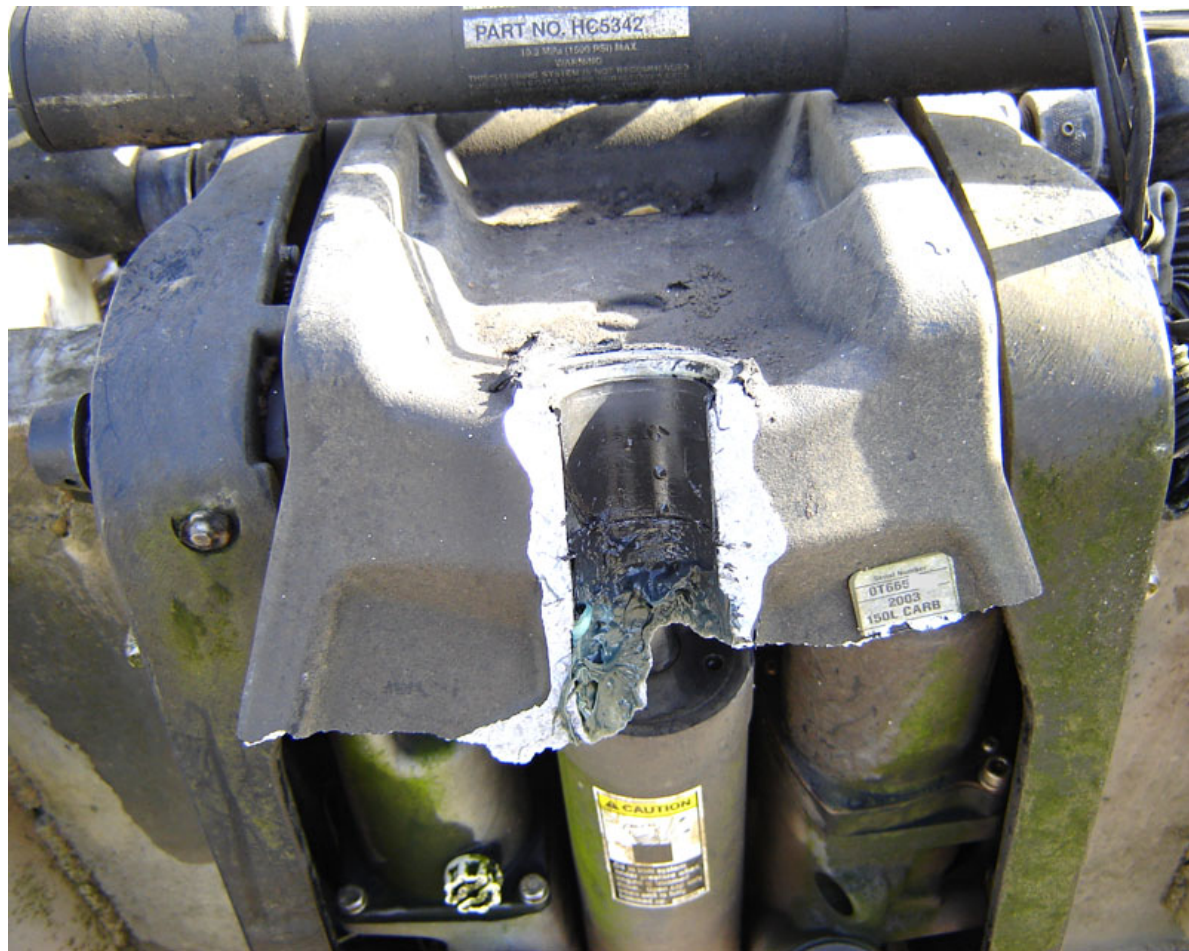
Figure 17: Failed swivel bracket 150 horsepower Mercury Marine closeup
