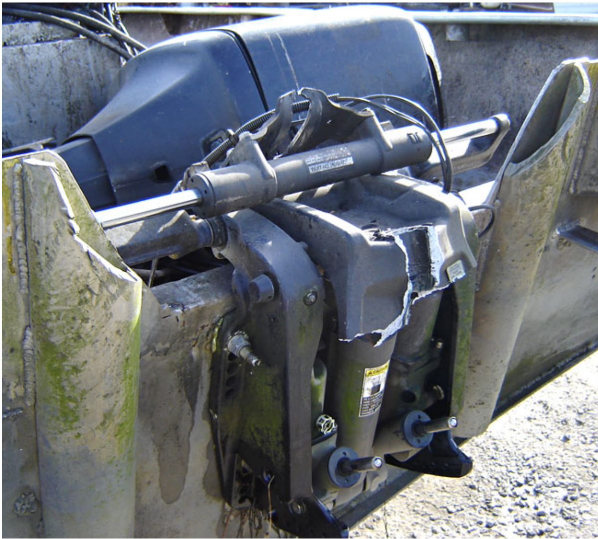
Figure 16: Failed swivel bracket 150 horsepower Mercury Marine
