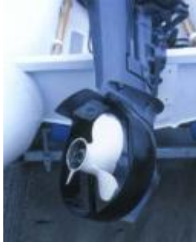
Figure 5.2 Ring guard incorporating a Kort Nozzle 6
