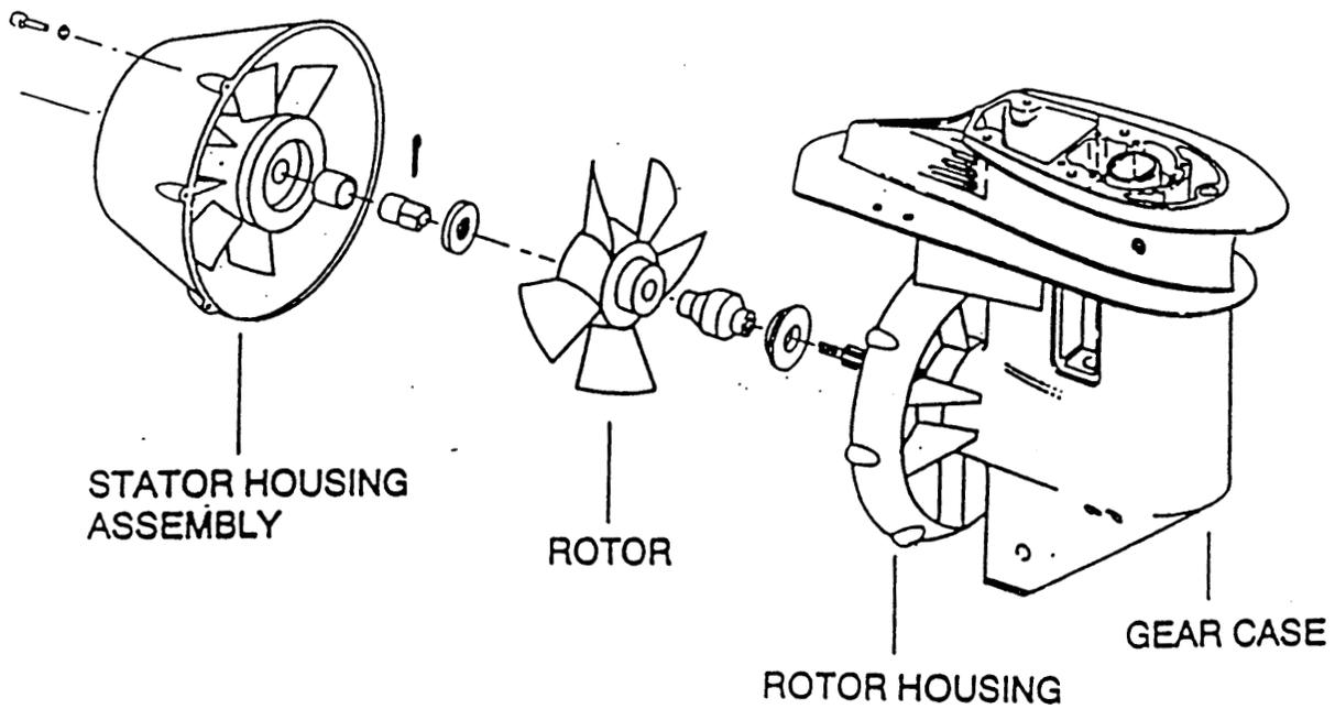
Figure 2. Pump Jet Propulsion Assembly for MARS Motor
