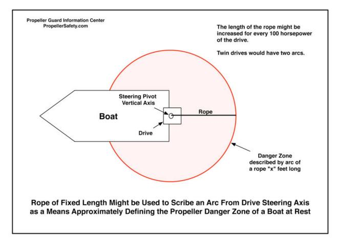
We suggest the "rope method" in the chart above as a place to start a discussion for possible ways to define the propeller danger zone. The arc traveled by a rope "x" feet long with one end held directly above the pivot point of the stern drive or outboard and the other end stretched out and held an equal distance above the water creates a symmetrical danger field. "Y" feet could be added to the rope for each additional 100
