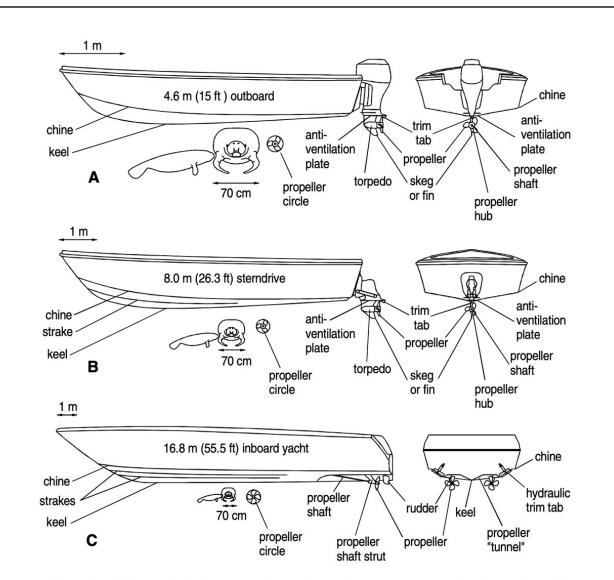
*Figure 2.* Watercraft hulls, propulsion units, and structures extending from them that can inflict wounds on manatees. A, B, and C watercraft with lengths of 4.6 m (15 ft), 8 m (26.3 ft), and 16.8 m (55.5 ft), respectively. An adult manatee (70 cm [27.6 in.] in diameter) with a nursing calf (130 cm [51.2 in.] in length) are illustrated in each drawing to provide scale for each of the watercraft and propellers shown.
